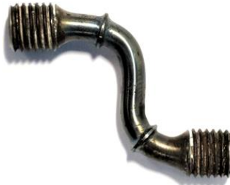
Figure 43: RLH10259 specimen that buckled under compressive loading using the load reversal cage
