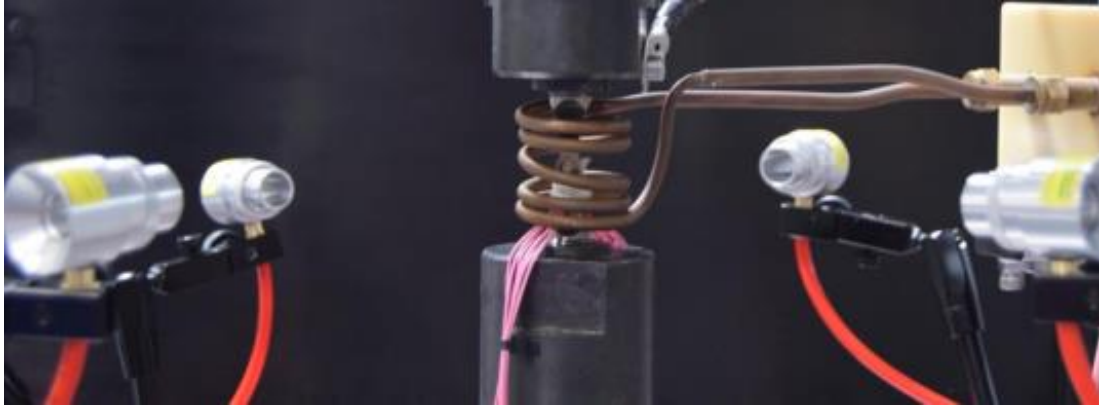
Figure 5.17 Image of the original implementation of air amplifiers. Each air amplifier has a separate compressed air feed and is held in position with an adjustable magnetic arm
