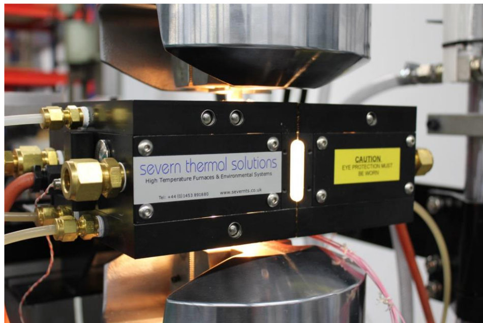
Figure 5.13 Image of the RLF setup adapted for the use of TMFCG testing
