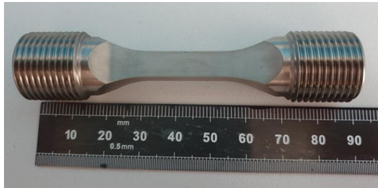
Figure 4.5 Image of Ti-6246 7x7mm corner crack specimens used throughout investigation
