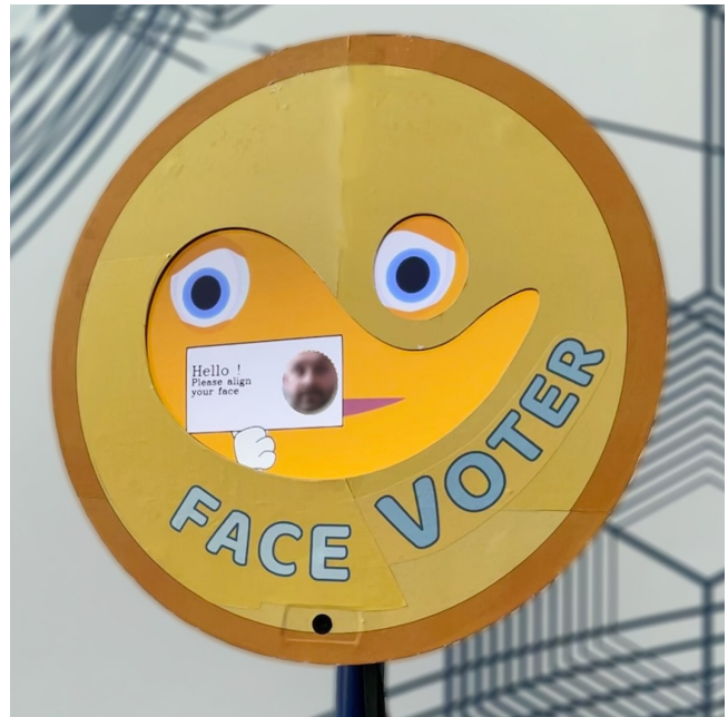
Figure 6: The FaceVoter prototype. Approaching the device, a user’s face is detected and the screen prompts them to answer Yes or No to a question by smiling or frowning.
