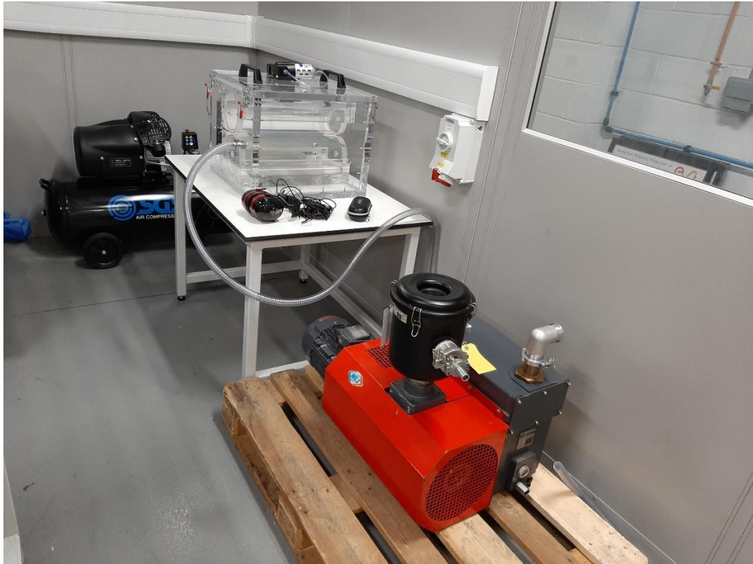
Figure 132: Vacuum lock experiment with vacuum pump and compressor
