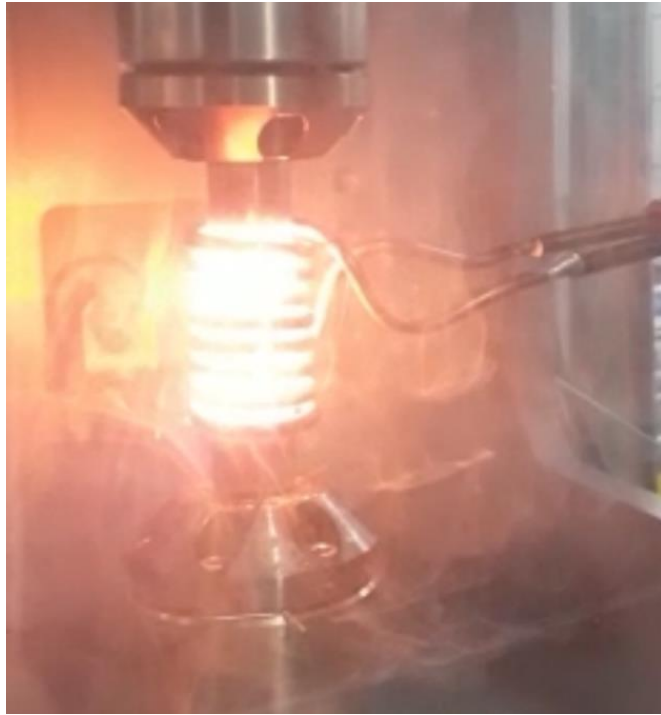
Figure 98 - Photograph of the tungsten platens and specimen at temperature prior to compression.
