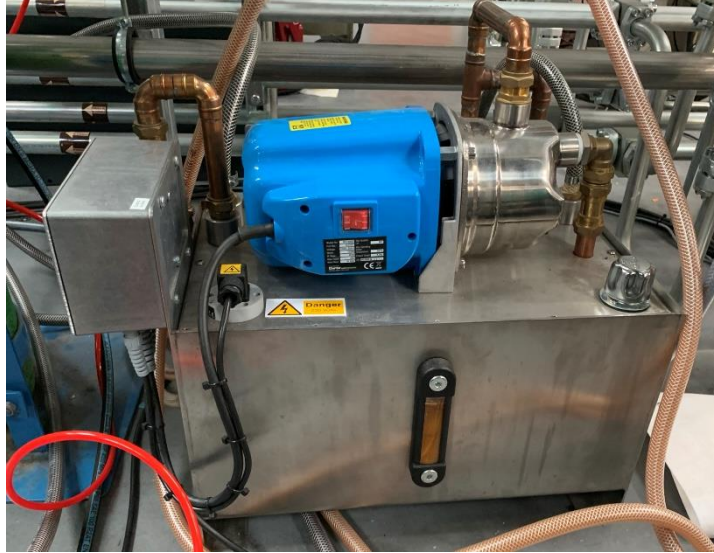
Figure 58 - Water-to-water heat exchanger with isolated distilled water reservoir for induction heater cooling.
