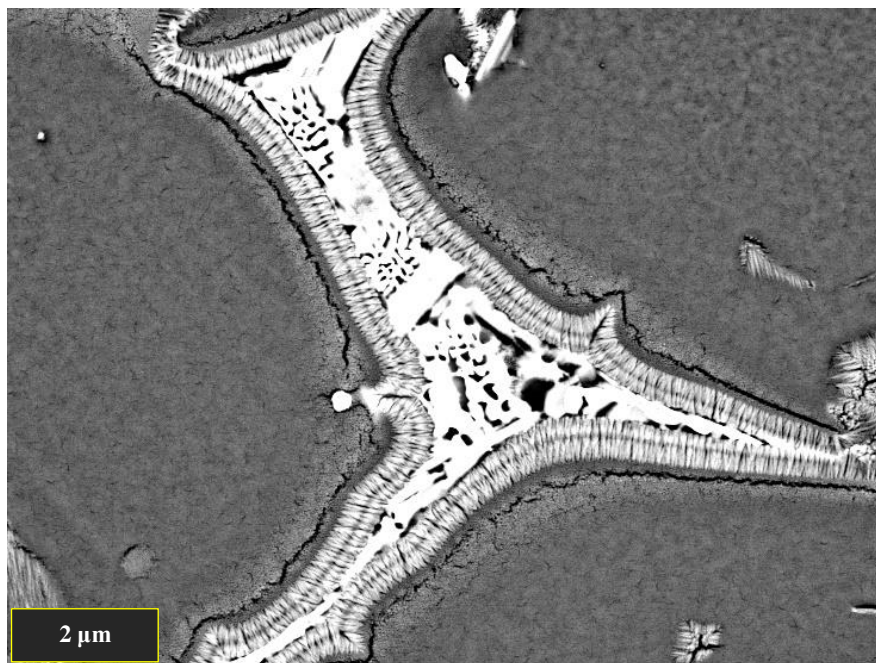
Figure 172 – BSE SEM micrograph of a eutectic feature formed on re-solidification of liquated material.
