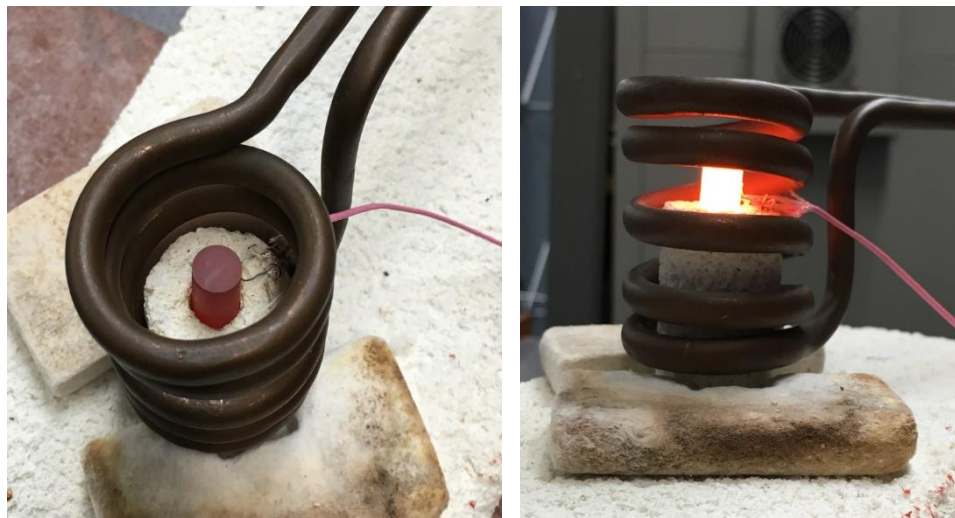
Figure 47 - RR1000 specimen with a spot-welded N-type thermocouple being heated to 1300°C with a 2kW induction heater.
