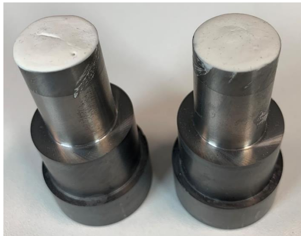
Figure 94 - Tungsten compression platens coated in ATP-9.
