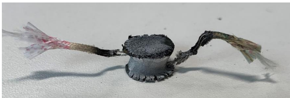
Figure 99 - Macro image of the CG specimen used in the first proof of concept test exhibiting inhomogeneous deformation at the top and bottom surface.
