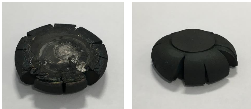
Figure 61 - 14mm diameter by 21mm height FG RR1000 compression specimen used in first trial run, exhibiting inhomogeneous deformation due to a temperature gradient during heating.
