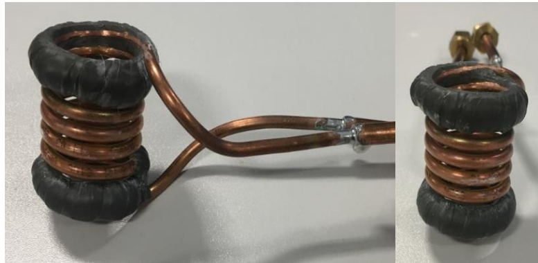
Figure 84 - Coil 13 featuring Fluxtrol applied to the first and last two turns of the coil.
