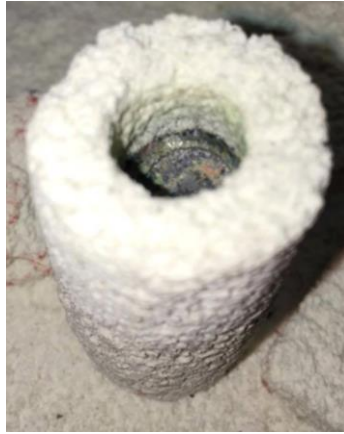
Figure 46 - Liquated RR1000 compression cylinder.
