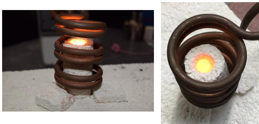
Figure 45 - 2kW easy heat induction heater trials set up.
