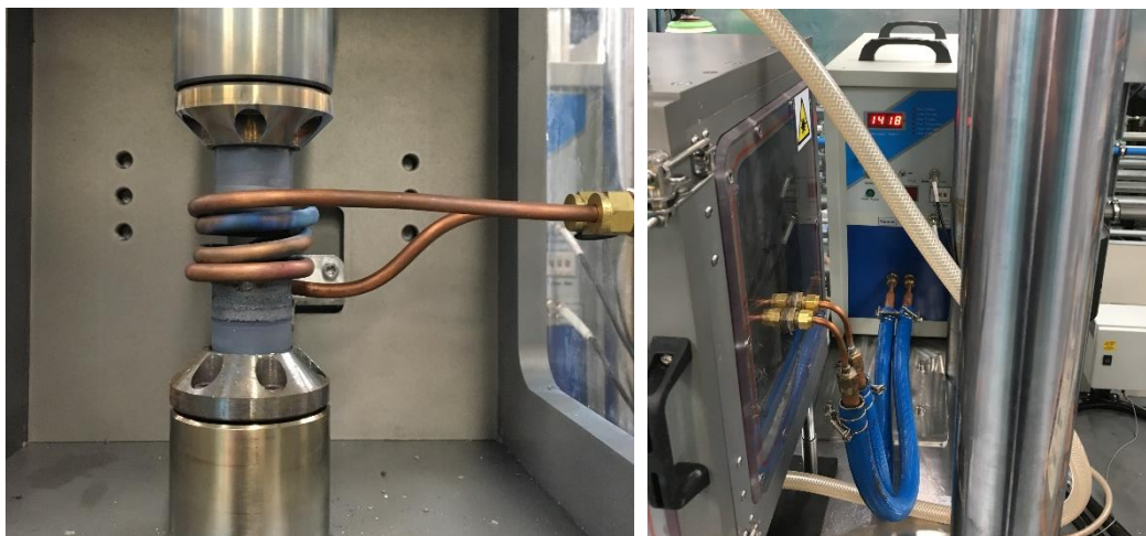
Figure 56 - JKZ induction heater configuration within the FG1 test frame.
