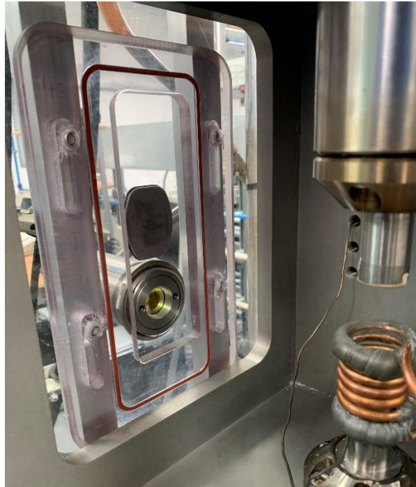
Figure 57 - Optris 3MH2 infrared thermometer mounted on a sliding Perspex panel at the side of the chamber.
