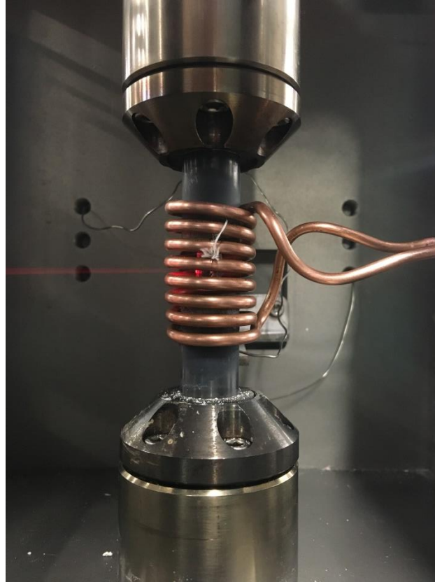
Figure 83 - A photograph of coil 12 with a 'floating' specimen within it and the tungsten platens inserted ready for testing.
