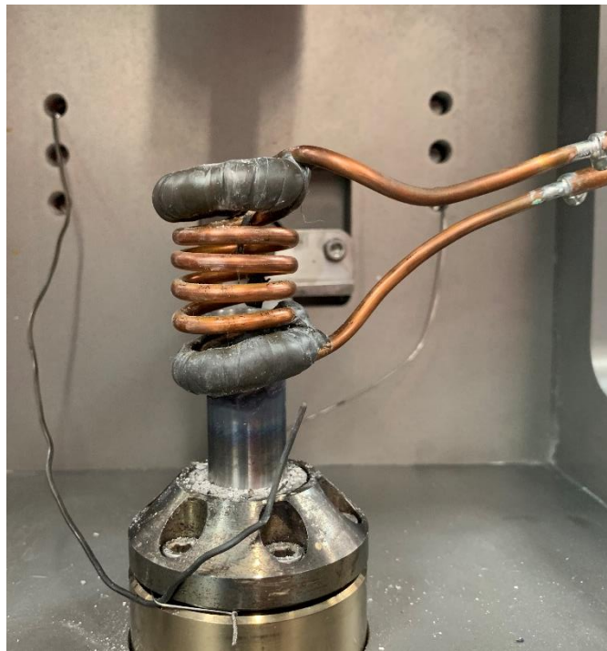
Figure 100 - Coil 13 after sustaining damage due to molten glass lubricant fusing the coil to the lower platen.
