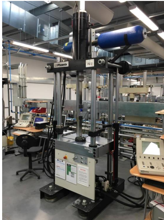
Figure 50 - FG1 Servo hydraulic compression machine to be modified for semi solid compression testing.
