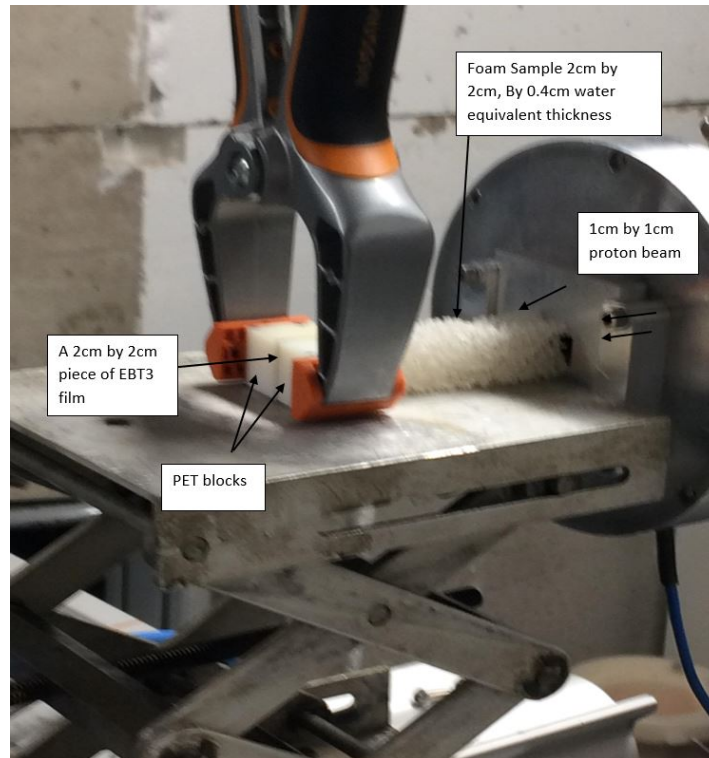
Figure 4.12: Experimental set-up used to measure variation in proton range due to variable bone structure and density. A piece of EBT3 film is placed perpendicular to the beam direction, clamped between pieces of PET block in front of the bone foam sample.
