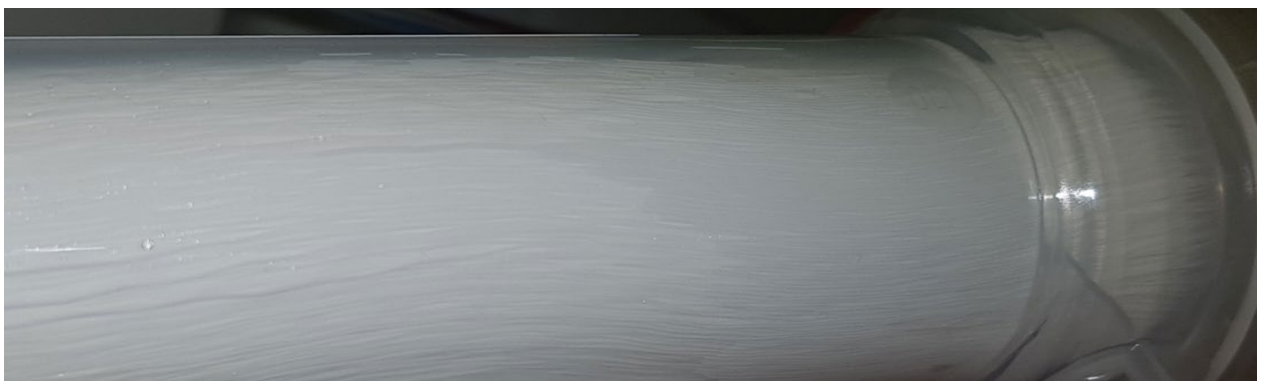
Figure 1.2 Polysulfone (PSU) high-flux dialysis membrane, following a dialysis session and a rinse with 360mls of dialysate fluid.
