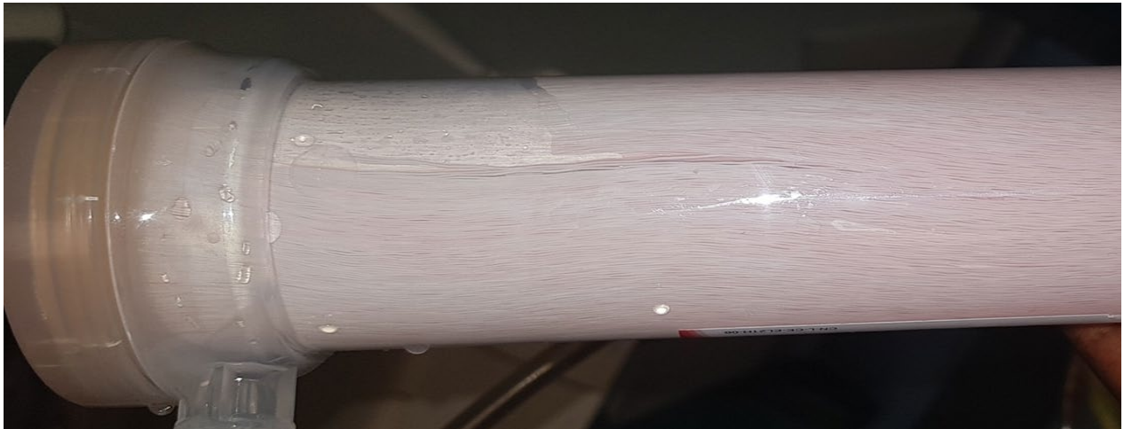
Figure 1.1 Polynephron membrane (second generation high – flux polyethersulfone (PESU)membrane) picture taken following a dialysis session and rinsing with 360mls of dialysate fluid.
