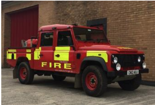
One of Four Land Rover 130 Crew cabs used to tow Argocat off road vehicles and firefight off road
