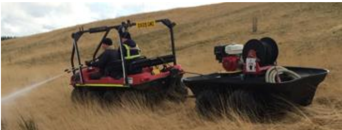
Argocat 8x8 complete with off road trailer and fire fogging system capable of transporting 4 firefighters
