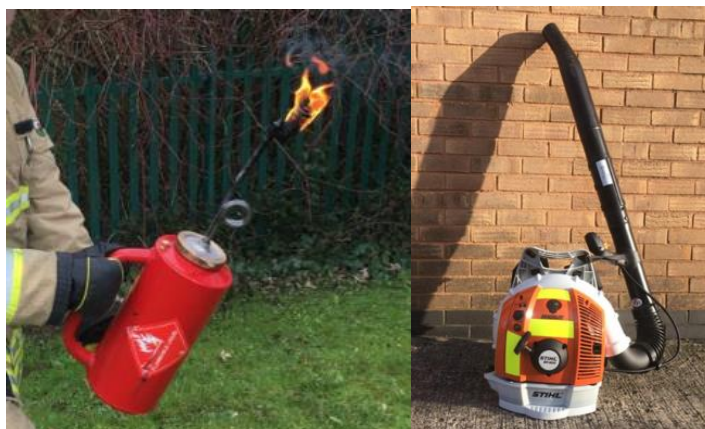
Drip torch containing 75% diesel and 25% petrol used for igniting prescribed and tactical fires, Stihl Br600 leaf blower used alongside a fire beater to extinguish fire, new equipment for SWFRS Photo credit- author
