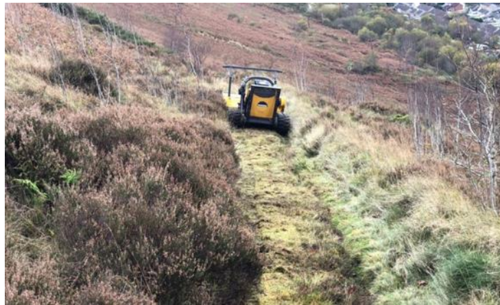
McConnell robo cutter used to create fire breaks across South wales
