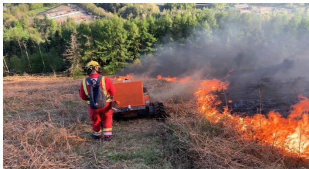
Firefighter operating a remote control cutter to create a fire break and stop a wildfire, Wattsville, South wales, April 2018 Photo credit - author
