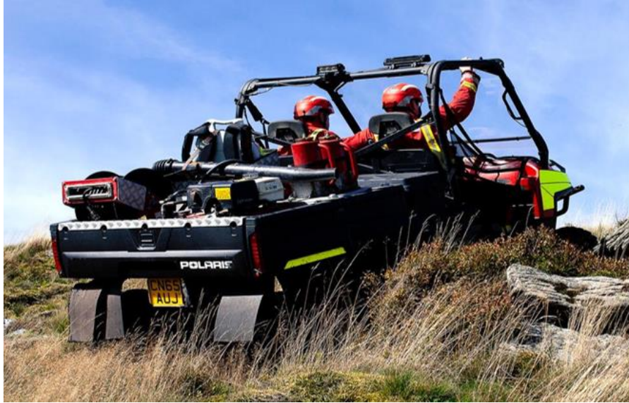
Polaris avenger 6x6 equipped for firefighting, note innovative stowage of fire beaters also acting as mud flaps
