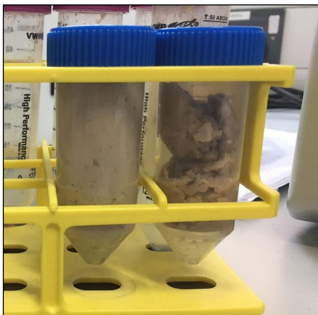
Figure 5.0: A visual comparison of the Omni homogenisation technique (left) and a standard hand blender technique (right)
