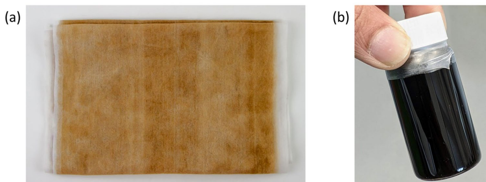
Fig. 1 a Photograph of a section of face mask material used for CNT production. Sections were cut and b dispersed in toluene to form the plastic carbon precursor seen in a vial
