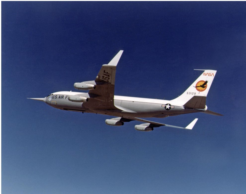
Figure 4: KC-135A Stratotanker flight testing winglets in 1979. Image EC79-11314, Dryden Flight Research Center Photo Collection, NASA[3]
