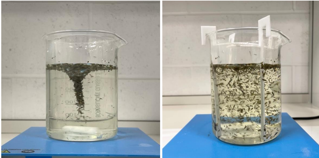
Figure 20. Mixing pattern without (left) and with baffles (right)
