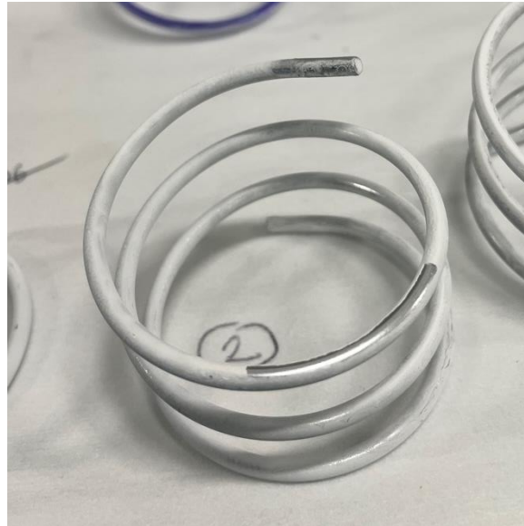
Figure 47. Material stripped through dip coating due to piling.
