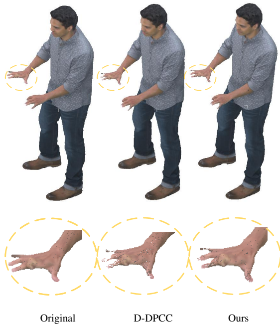
Fig. 12. Visual comparison of frame reconstruction between D-DPCC and our method, based on the 30th frame of the Loot point cloud sequence, which contains 779986 points. The compression rate is set to 0.25 bpp. D1-PSNR of D-DPCC and our method are 75.6 and 76, respectively.
