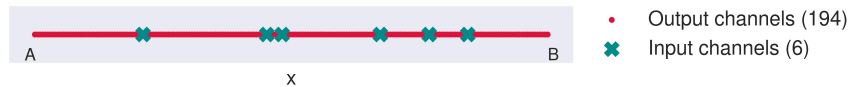
FIG. 9: The 1D grid used to generate the Ground Truth (GT) for 1D transient heat conduction. The input and output channels of the mesh nodes are highlighted, with the six green crosses being the input channels and the 194 red dots being the output channels. The temperature values at the six input channels are given to the ML model, whereas the temperature values at the 194 output channels are generated by the ML model at every time step, which is equal to 1s in this case. The locations of the six input channels are randomly selected.
