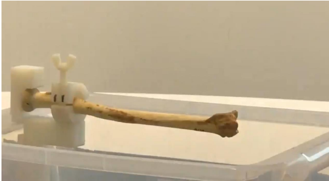
Figure 3.2.2.1.2.1. Final suspension bracket design
