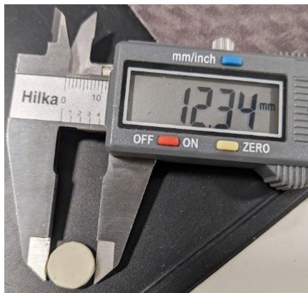
**Figure 3.9.3** – Sopac20-HRc-Bo 12mm disk prepared for LFA analysis. The coating disk was prepared specifically for this technique and was machined using a Dremel 3000 rotary tool.
