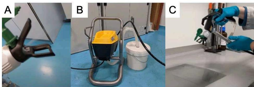
**Figure 5.29** a) Air-spray nozzle utilised for initial viability application trials b) Spray system’s pump and coating reservoir c) Application of Sopac20-HRc-HBo to sheet steel.
