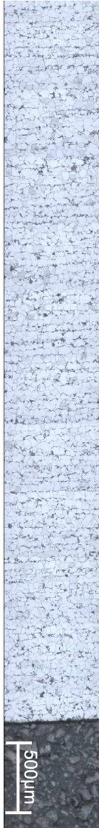
**Figure 3.4.2** –Cross-sectional Vertical Stitch at 200X magnification for a Grain Size analysis of Sopac20 coated E1 Steel.
