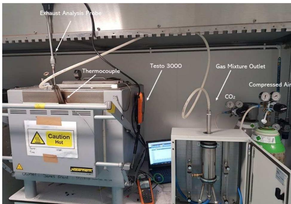
**Figure 3.1.4** – Overview of the Atmospheric Furnace rig in PMRC. The rig consists of gas bottles, mixing mechanism, probe apparatus and a box furnace.
