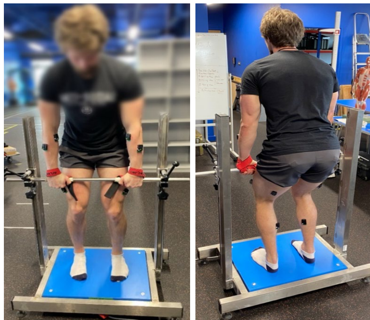
Figure 3.2 Anterior (left) and posterior (right) view of a participant in the IMTP position, equipped with sEMG sensors, prior to the initiation of the pull.
