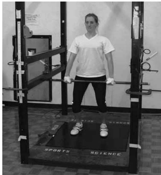
Figure 2.10 The custom designed isometric testing rack placed over force platforms, using a combination of pins and hydraulic jacks to fix the bar at the appropriate height with respect to the participant. From, Relationship Between Strength Characteristics and Unweighted and Weighted Vertical Jump Height - Scientific Figure on ResearchGate . Available from: https://www.researchgate.net/figure/Isometric-mid-thigh-clean-pull-testing-Top-schematic-isometric-mid-thigh-clean-pulls_fig1_40759599 (Kraska et al., 2009). Similar setup as the one previously used in seminal research (Haff et al., 1997, 2005).
