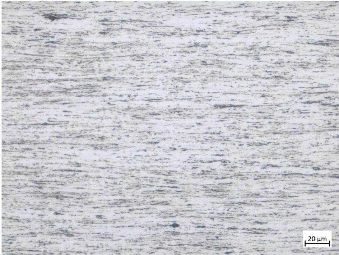
Figure 9.1. Optical image of nitrogenised grade 3465, in its transverse orientation, in its cold rolled condition at a magnification of 500x.
