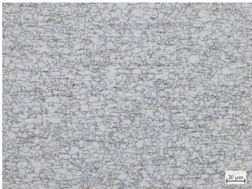
Figure 9.5. Microstructure of 3465 in its annealed condition when heating rate=200°C/s and soak temperature=635°C.
