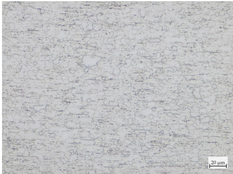
Figure 9.4. Microstructure of 3465 in its annealed condition when heating rate=20°C/s and soak temperature=635°C.
