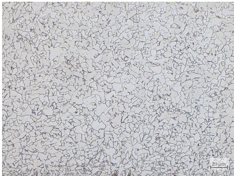
Figure 9.7. microstructure of 3465 in its annealed condition when heating rate=20°C/s and soak temperature=850°C.
