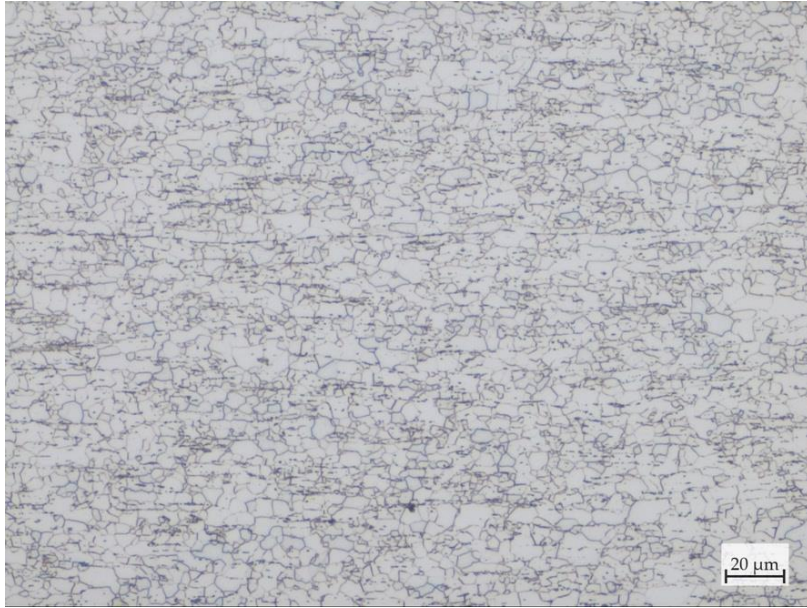
Figure 9.6. Microstructure of 3465 in its annealed condition when heating rate=1,000°C/s and soak temperature=635°C.
