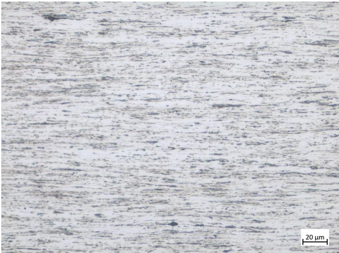
Figure 3.1. Optical image of nitrogenised grade 3465, in its transverse orientation, in its cold rolled condition at a magnification of 500x.
