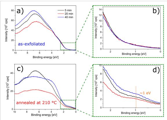
**Figure 4.** (a) Valence band of the ANS samples obtained by ultrasonication for 5, 20 and 40 min measured by ultraviolet photoelectron spectroscopy (UPS). (b) Enlarged view of the square-dashed area in (a). (c) Valence band of the same samples in (a) after annealing at 210 °C. (d) Enlarged view of the green-dashed area in (c) showing a peak near 1 eV ascribed to antimonene oxide. The Fermi level located at 0 eV.
