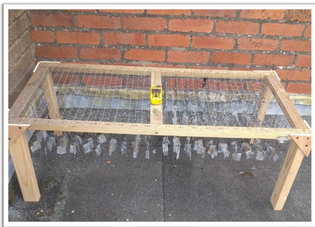
Fig. 6. Test rack for natural weathering showing suspended samples
