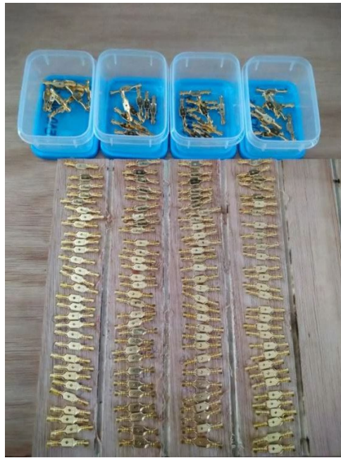
Fig. 5. The prepared brass spade connectors
