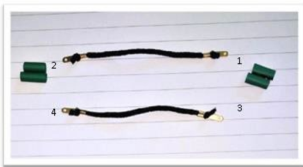
Fig. 7. Assembly of the harness, showing the order in which the ends were connected to balance tension.
