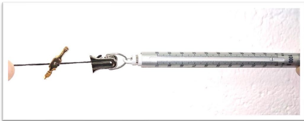
Fig. 4. Tying knot to tension using Pesola scale as dynamometer.
