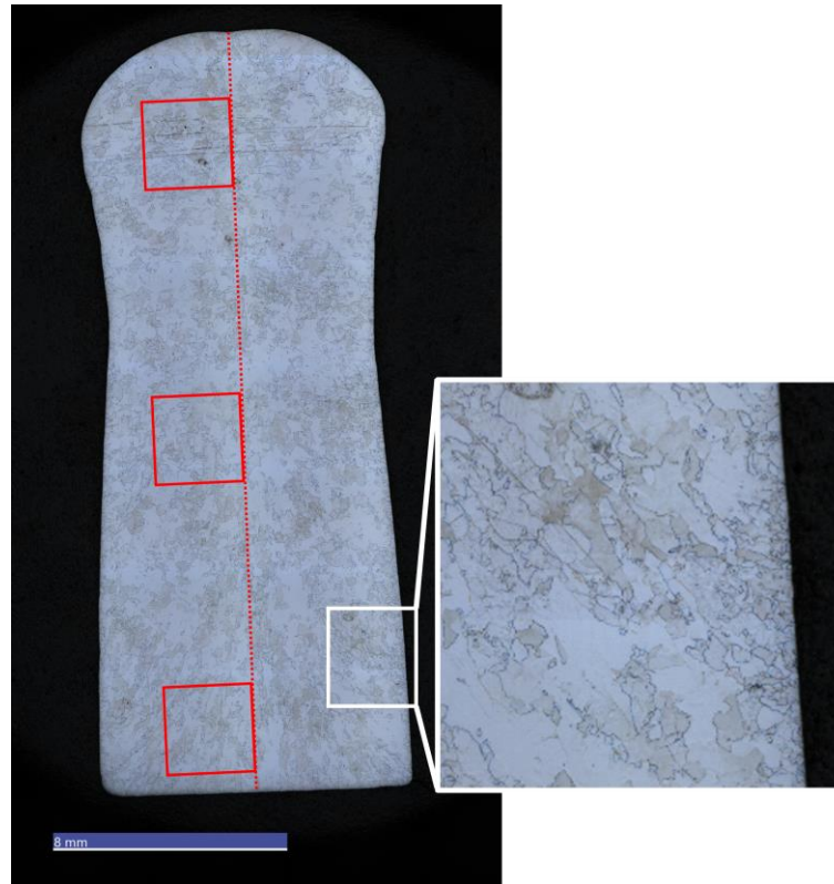
Fig. 62 – Microstructure of the RAP 80g IF remelted as-cast sectioned in the Z-Y plane in reference to Fig. 34.
