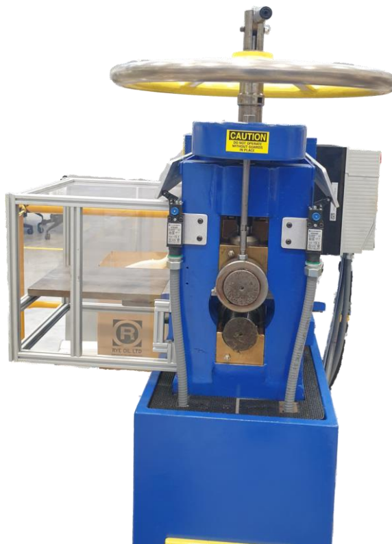
Fig. 20 – Small cold rolling mill.
