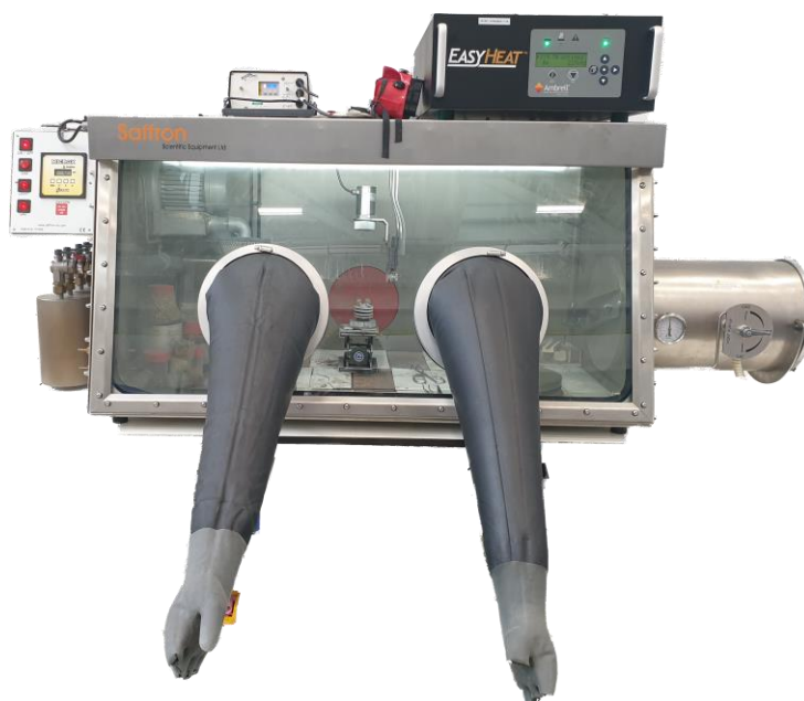
Fig. 12 – Coil Induction Melting (CIM) glovebox for 40-80g of material.
