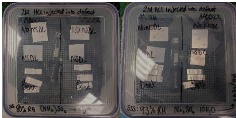
Figure 7.2d: Sealed boxes containing both flat and bent samples at 80% RH (Ammonium Sulfate) and 93% RH (Sodium sulfate Decahydrate)
