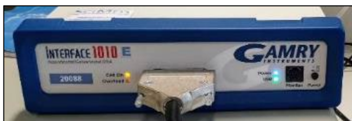
Figure 2.5.2a: Gamry instruments interface 1010E used to take open circuit potential, OCP, and potentiodynamic measurements
