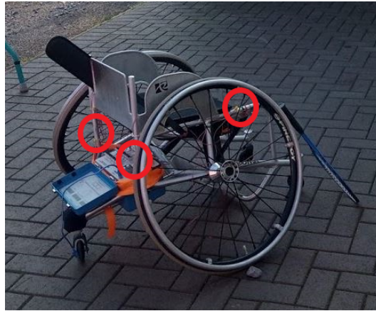
(a) Strain gauged RMA sports tennis wheelchair(strain gauge locations marked in red)
