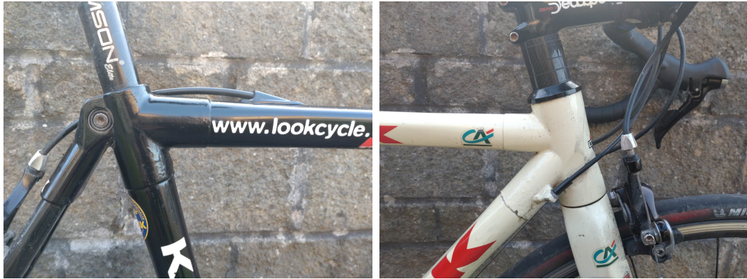
Figure 2.16: The 2003 Look KG381 road bike frame uses carbon tubes bonded to aluminium lugs
