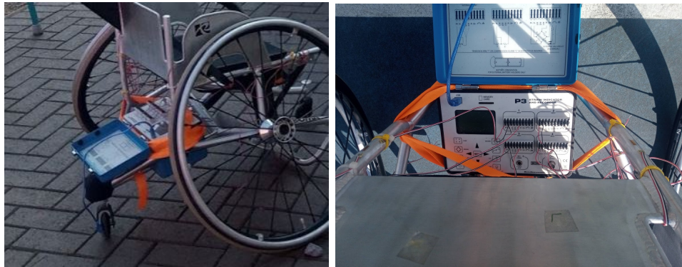
(a) P3 data logger (View 1)
