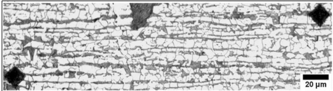
Figure 11 Example of a banded dual phase microstructure [59]
