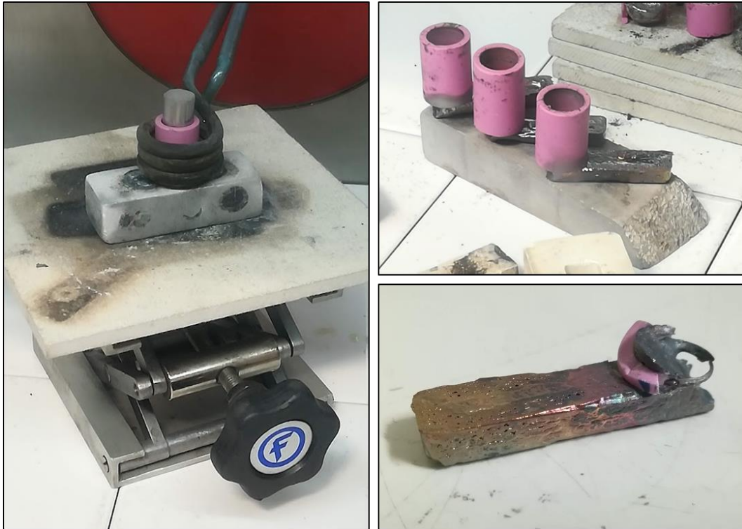
Figure 18 Images of the melting setup and resulting bar casts from the 20g method, showing a powder compaction in a crucible in the induction coil and four bar casts
