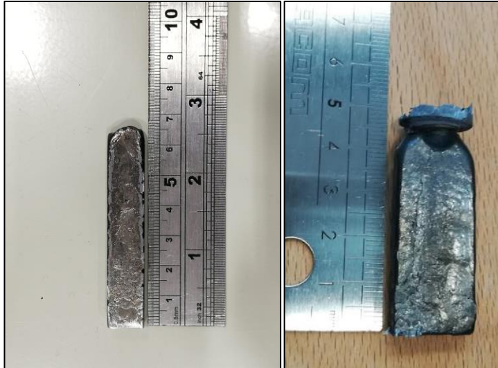
Figure 27 40g cast from the initial mould trials (left), and the subsequent wider bar cast from a later mould (right)
