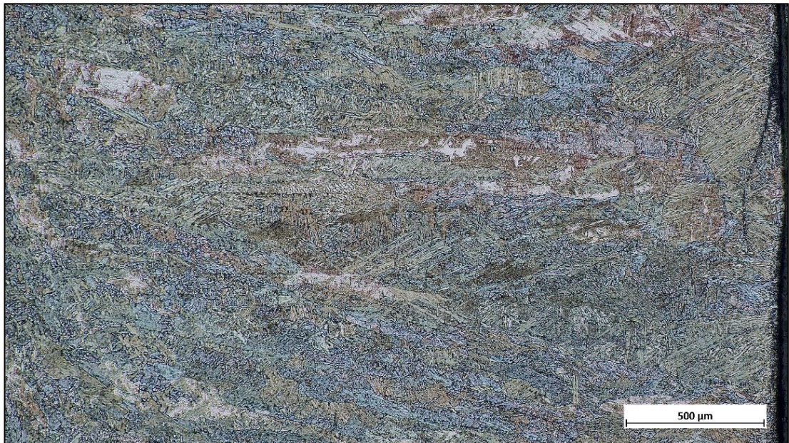
Figure 132 Optical image of the as-cast microstructure in RAP40G_MA_SOL_RF showing the edge of the sample in the narrower plane
