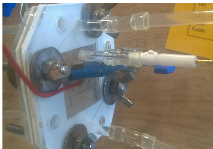
FIGURE 4.18: Photo showing the inclusion of a reference electrode on the MK 2 cell.
