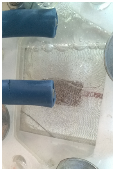
FIGURE 4.17: Photo of the MK 2 cell showing the visibility inside the cell and anodic gas build up.
