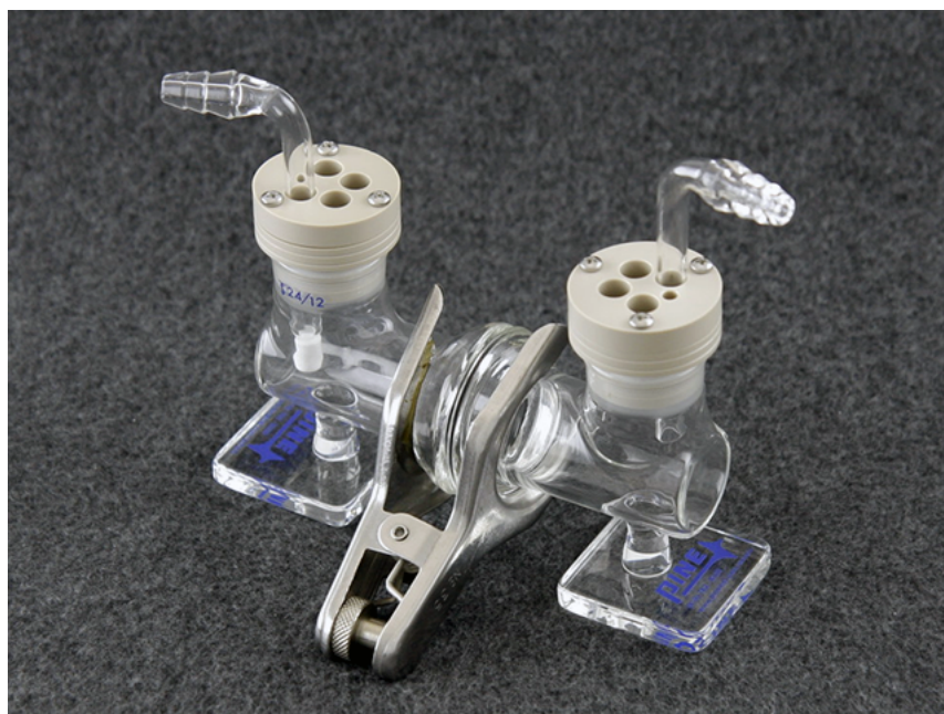
FIGURE 4.2: Photograph of the Pine Research Low Volume Separated Cell [97].
