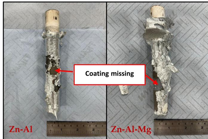
Figure 29. Visual inspection of the bar specimens tested in Zn-Al (left) and Zn-Al-Mg (right).
