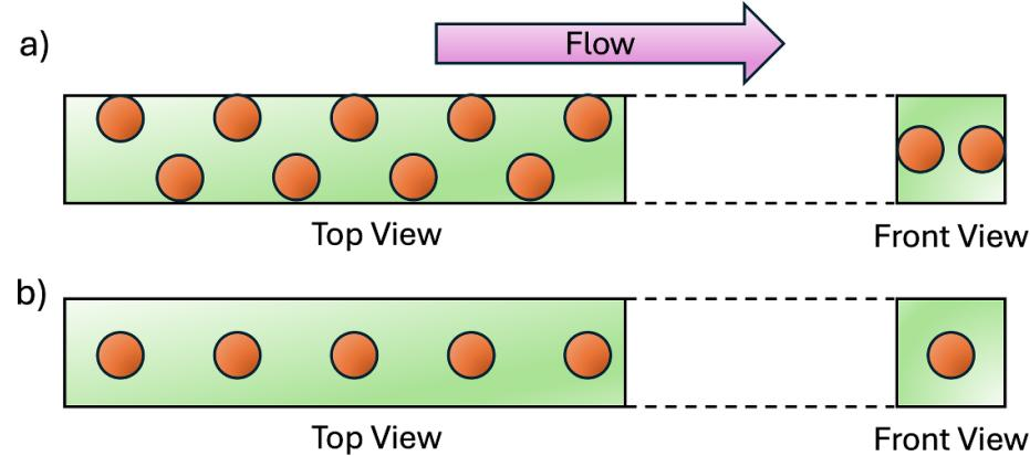
**Figure 1.** Schematic representation of ordering in microfluidic devices for (a) inertial flow and (b) viscoelastic flow.
