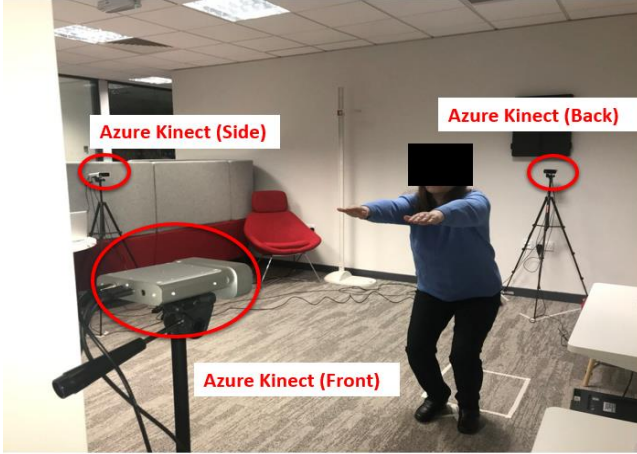
Figure 1: Overview of the entire setup. Participant performing deep squat while three MS Azure Kinects are capturing the motion.
