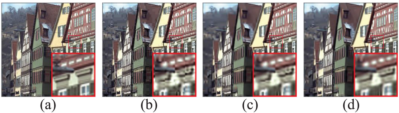
FIGURE 7 Visualization of image buildings in the LIVE1 dataset (image size: 256 \times 256 ) under compression quality Q = 10 deblocked by various algorithms: (a) Original image, (b) JPEG compressed image (PSNR = 23.83 dB, SSIM = 0.8232), (c) SA-DCT (PSNR = 24.66 dB, SSIM = 0.8177), and (d) the proposed algorithm (PSNR = 25.11 dB, SSIM = 0.8311).
