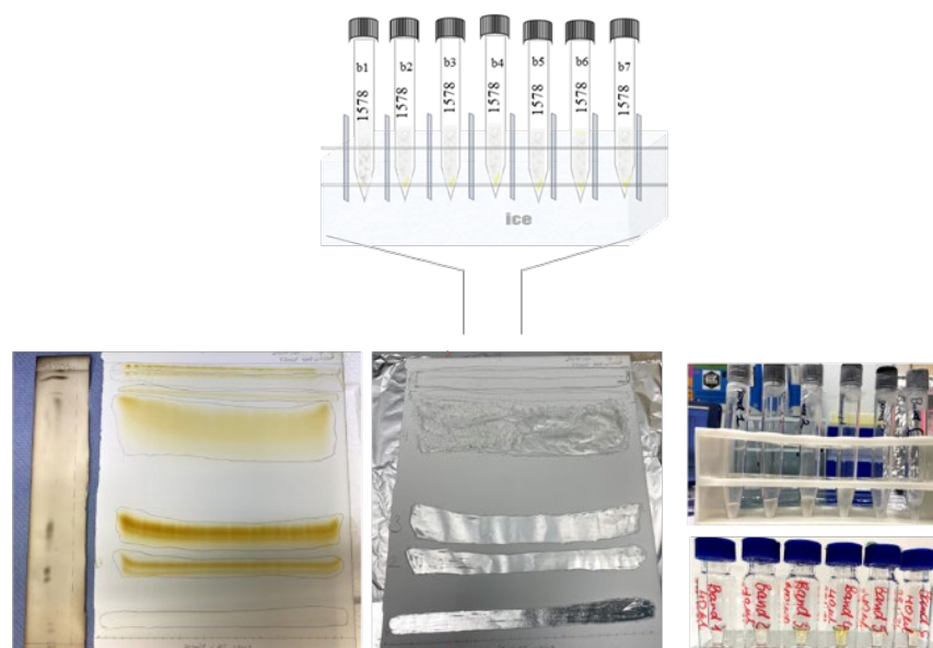
Figure 3:7: Example of preparative TLC – staining and scraping of discrete lipid bands into glass tubes and then preserved overnight in 1 ml methanol at -20°C, ready for further processing the next day.
