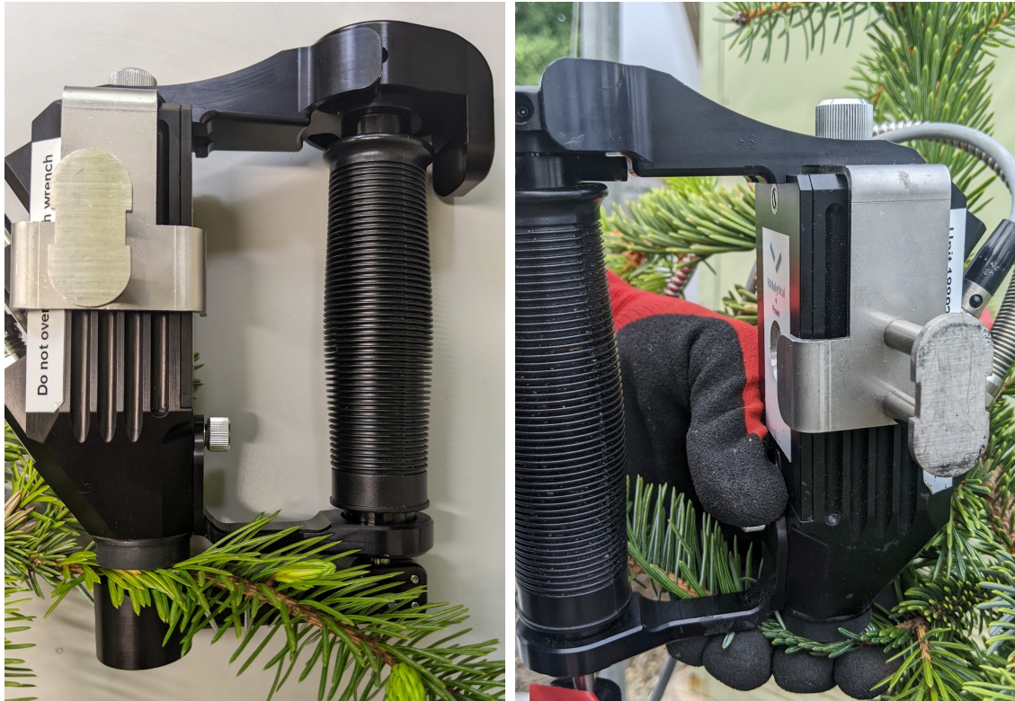
Figure 2.1: Measuring Sitka spruce spectra in situ on a branch. Left image: Using the leaf clip without a glove creates gaps between the contact probe and the sample (seen by the light escaping above the sample, also see Appendix A, Figure A.1 (p.176)). Right image: with the introduction of a low reflectance glove the user is able to apply pressure to the sample which facilitates a greater contact between the sample and probe.
