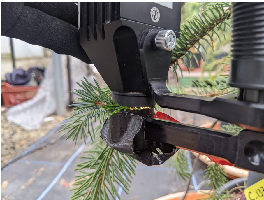
Figure A.1: The standard leaf clip for spectral measurements using a field spectroradiometer (ASD FieldSpec 4 standard Res, Analytik Ltd, Cambridge). The leaf clip is designed for flat, broadleaf plants. When recording in situ conifer needles light escapes, potentially confounding spectral measurements.
