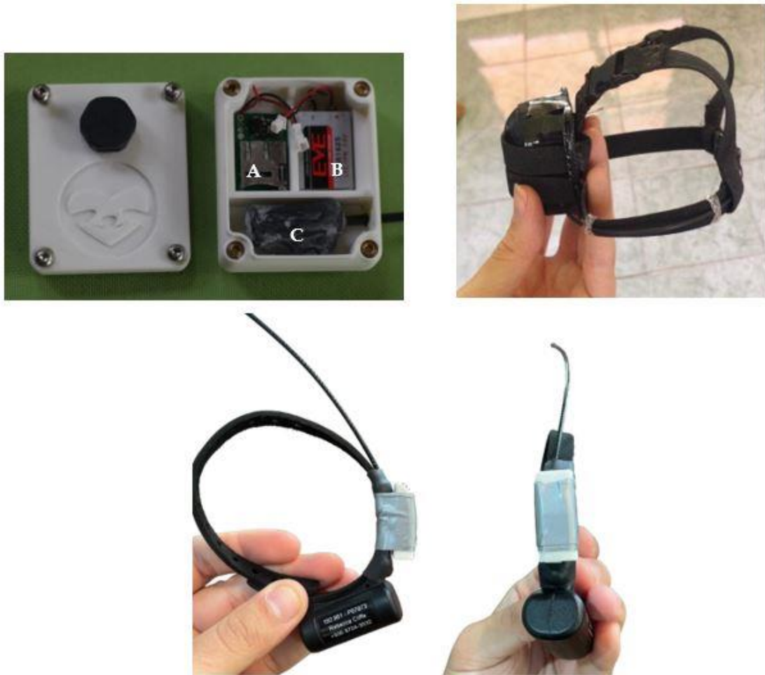
Figure 3. Top left panel: 3D printed case measuring 4 cm x 5 cm 2cm with DD (A), battery (B) and VHF pip transmitter used in human-impacted forest (C). Top right panel: case and harness used in secondary forest (Cliffe et al. 2023). Bottom panel: Axy attached to VHF radio collar
