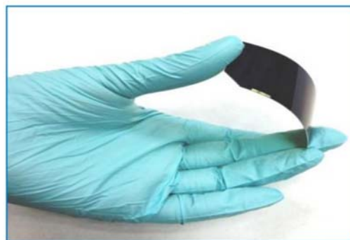
Fig. 2 Image of a CTJ30-80 solar cell in a curved arrangement [19]
