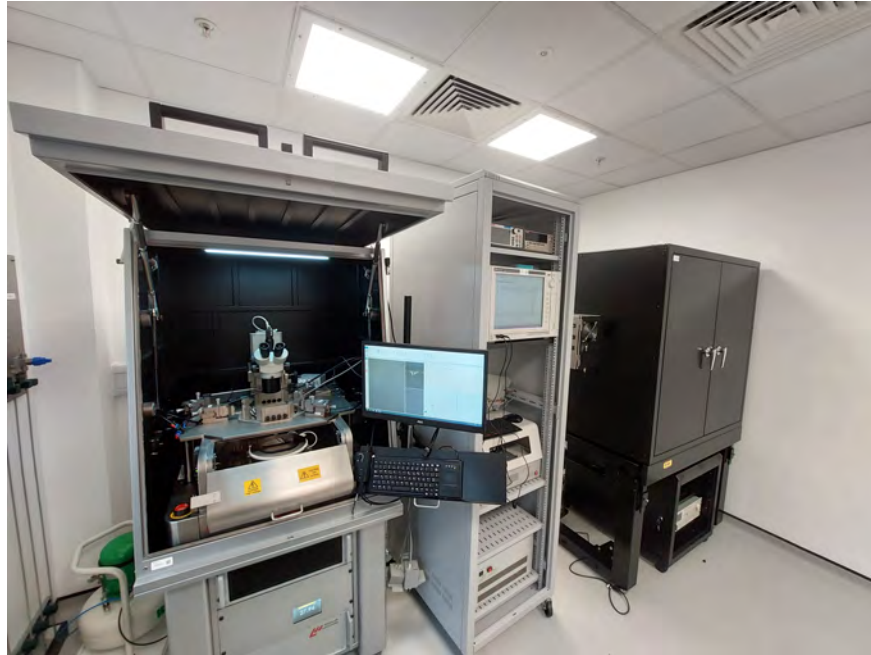
Fig. 5.5 Electrical test setup consisting of a Wentworth S200FA semi-automated probe station (left) and a Keysight B1505A Power Device Analyser (centre).
