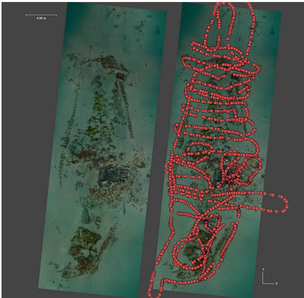
Figure 5. 2019 Post-excavation survey and improved survey pattern resulting in better coverage and image alignment.
