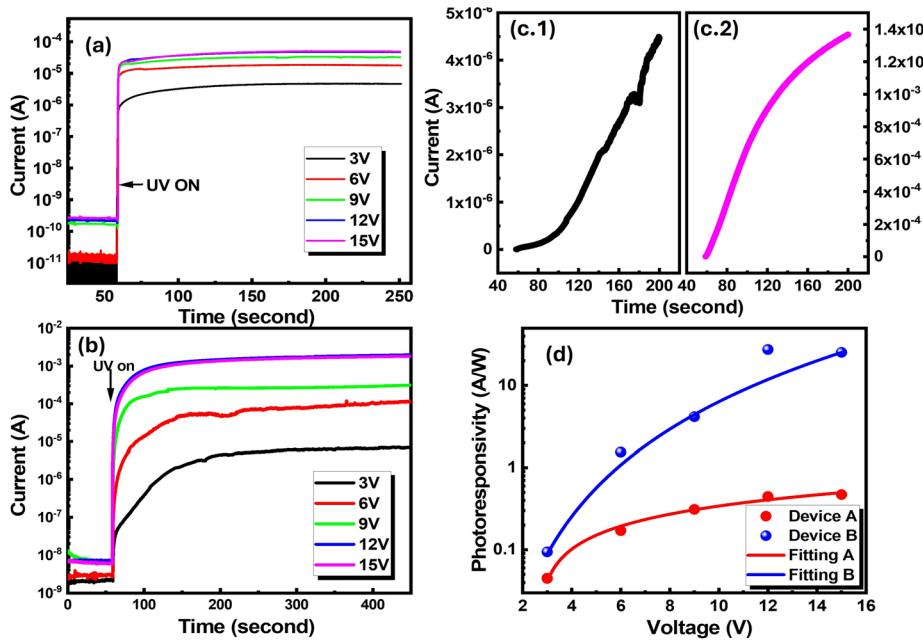
FIG. 3. The photocurrent rise measured under different voltages of devices A (a) and B (b), respectively. (c.1) and (c.2) show the linear plot of device B at 3 and 15 V. (d) Saturation photoresponsivity as a function of voltage for both devices.
