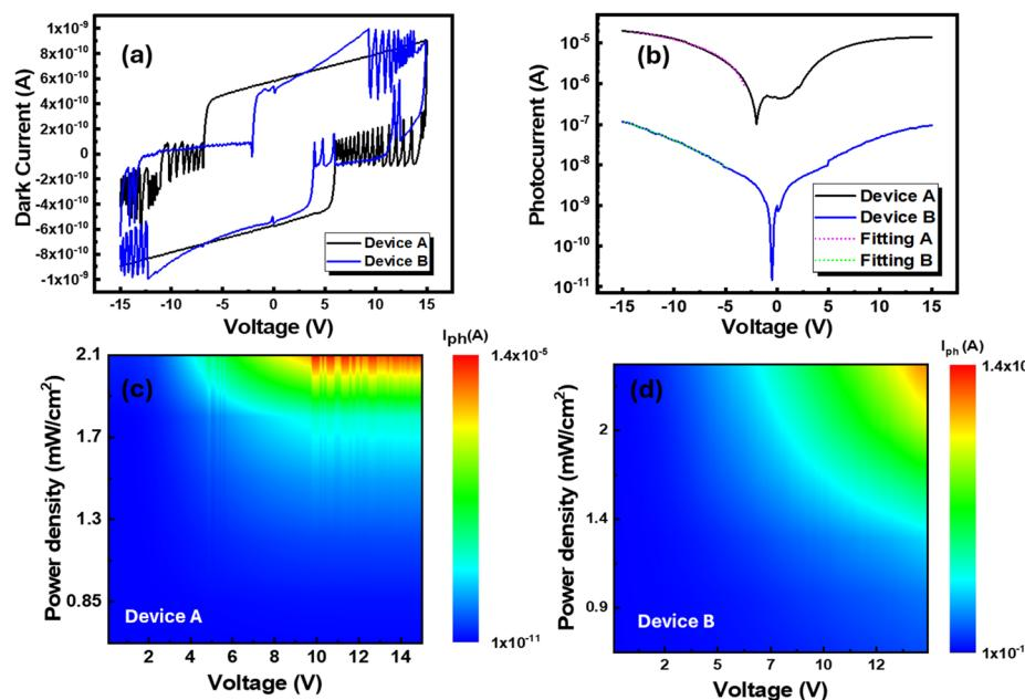
**FIG. 1.** (a) Dark current of the as-grown (device A) and annealed devices (device B). (b) The IV curve of both devices under UV254 illumination with power density of 2.1 and 3.1 mW/cm<sup>2</sup> for devices A and B. The photocurrent is limited by the sampling rate due to the long decay time. (c) and (d) Photocurrent mapping under different illumination densities of devices A and B, respectively.
