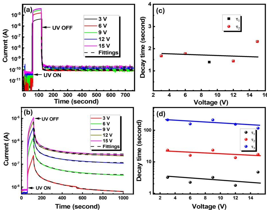
FIG. 2. Transient photoresponse of devices A (a) and B (c) at applied voltage from 3 to 15 V; the dashed lines are the fitting curves. (b) and (d) The time constant from the fitting of devices A and B, respectively.
