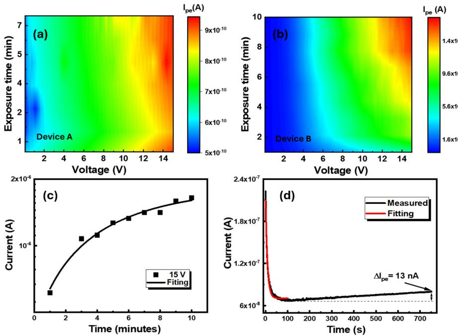
FIG. 4. The  $I_{pe}$  mapping of devices A (a) and B (b). (c)  $I_{pe}$  measured at 15 V under different DUV exposure times. (d) Transient  $I_{pe}$  after 10 min DUV exposure at 3 V.
