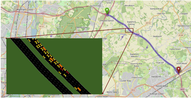
Fig. 10. Simulation of a cyber-induced vehicle disabling attack on a section of the M25 motorway, illustrating the resulting congestion and disruption to traffic flow.
