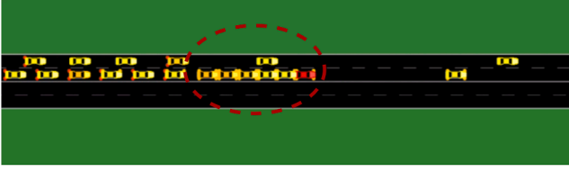
Fig. 8. Simulation of a cyber-induced sudden deceleration event leading to a multi-vehicle collision on a motorway, illustrating the propagation of secondary crashes due to traffic disruption.
