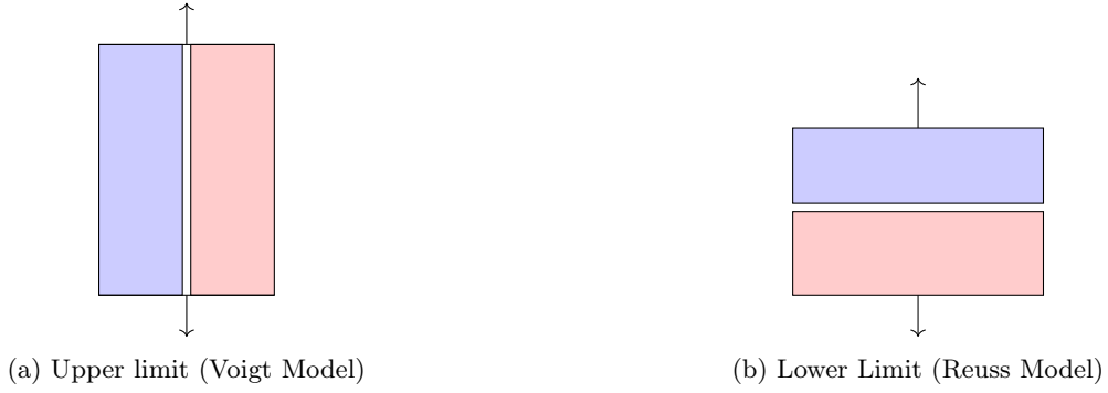
Figure 1.2: Parallel and series model for the elastic property limits of a composite material
