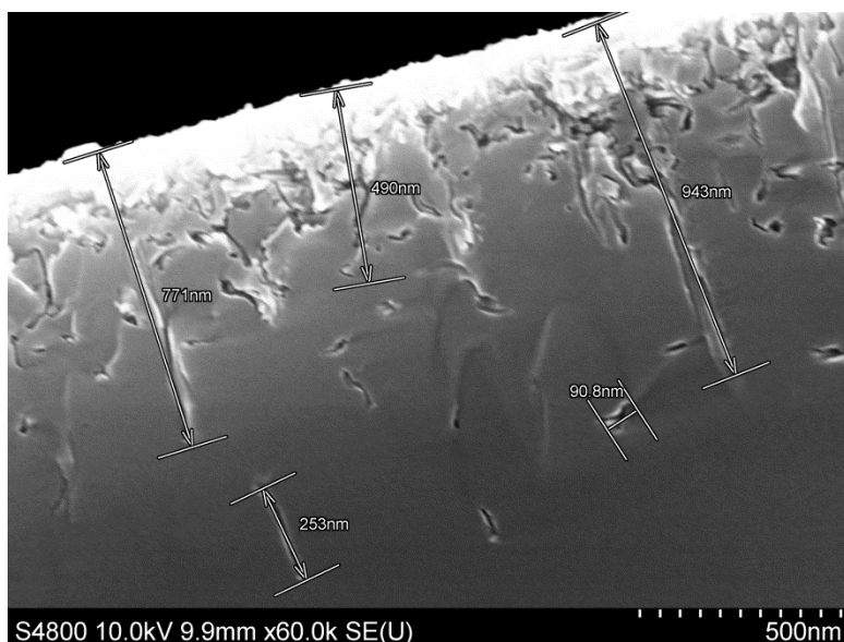
Figure 66: Cross-sectional image of 2 mins Metal-assisted etching of polished silicon substrate
