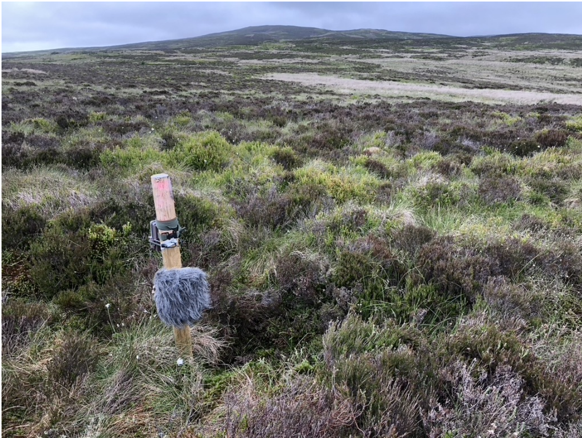
Figure 4.2: A Biophone Deployment. This shows deployment of the v1.0 device on the Cwm Hesgyn site with a furry hat cover over the top. Boxes were affixed to stakes in the ground with garden wire and screws and set to record.
