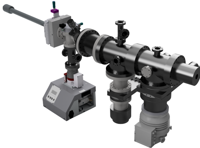
Figure 3.7: Illustration of the Full CAD model for the Caesium Sputtering Negative Ion Cluster Source
