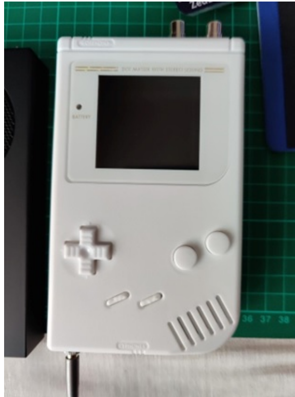
Figure 1. A modded Game Boy DMG containing a Prosound and 3.5mm auxiliary mod (photo provided by Price [author], July 2024).
