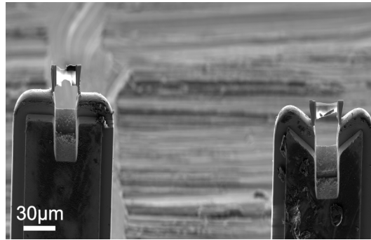
Figure 3.17: image showing the FIB lamellar cross section mounted ready for SEM analysis
