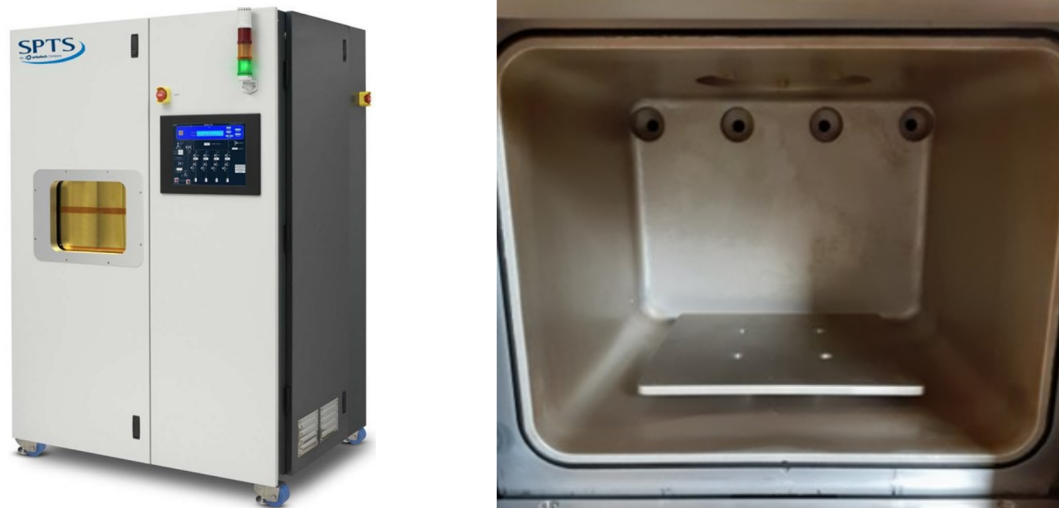
Figure 3.7: Image showing the MVD 300 by KLA and the exposed chamber in which the deposition takes place (right)
