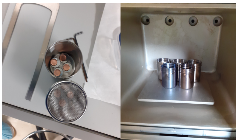
Figure 4.1: Image showing the experimental setup for how copper substrates were coated by MVD using stainless steel baffles to stop sample movement
