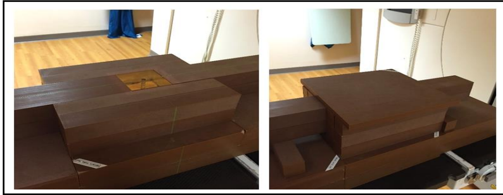
Figure 3.4: Photographs of the measurement setup with the microDiamond detector used during the investigations. A cubical phantom is being surrounded by a multi-block water-equivalent phantom to minimize the scattering effect (a) and two slabs of solid-water phantom equal to 1.5 cm thick is attached on top of the detector for measurement at 1.5 cm depth at SSD of 100 cm (b)
