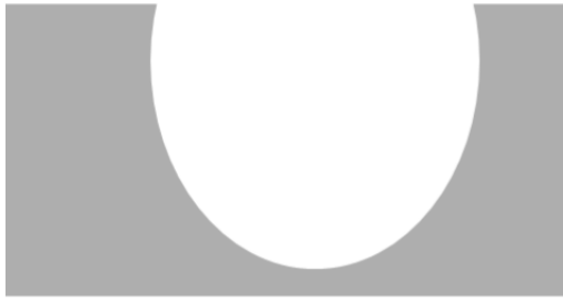
Figure 2.4: An isotropic etch profile Figure 2.5: An anisotropic etch profile
