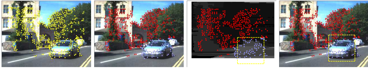
Figure 3: Left to right: sparse point tracking, foreground background segmentation and alignment with depth map, and final annotation.
